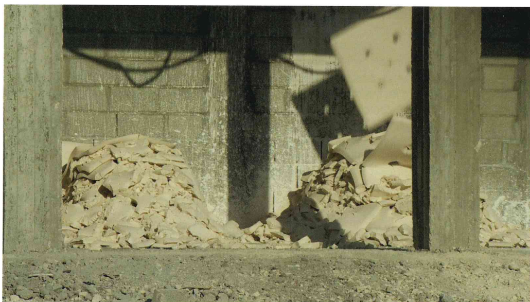
Production of dehydrated calcium carbonate in the al-Fahs plant with a humidity level of 12%
